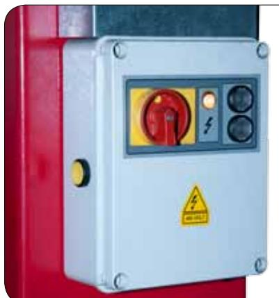
EN Automatic braking exclusion button. This function makes it possible to lower the lift without the initial upward step.
