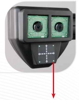
The integrated synoptic panel **with light indications** allows the operator to check the target hooking status and guides him/her through the various operational steps. During compensation and steering procedures, illuminated arrows provide clear information about the current procedure.
