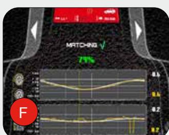
**LASER RUN-OUT MEASUREMENT:** The laser measuring sensors are also used to precisely calculate both radial and lateral tyre Run-Out. TECO 750 allows to identify the best tyre-rim coupling in order to maximize the driving comfort of the vehicle.
