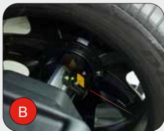
**LASER POINTER AND RIM ILLUMINATOR:** Standard with internal Laser pointer system and rim illuminator. If ALU programs are selected, the Laser pointer assists the operator during adhesive weight positioning. The rim illuminator supports operators during rim cleaning and weight application.
