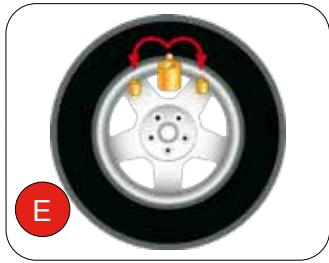
**HIDDEN WEIGHT AND SHIFT PLANE PROGRAMS (ALU P):** «Hidden Weight» subdivides the external adhesive weight in 2 parts to be positioned behind the spokes of the rim. The **patented** program «Shift Plane» calculates the balancing position to allow using commercial adhesive weights.
