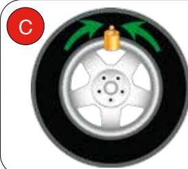
**(EN) AUTOMATIC BALANCING POSITION SEARCH:** Variable speed belt spin system to reduce operational noise and improve working lifetime and electronic shaft locking system. After the spin, the balancer automatically stops the wheel at the right weight application position.
