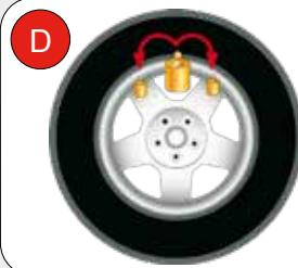
**(EN) HIDDEN WEIGHT AND SHIFT PLANE PROGRAMS (ALU P):** «Hidden Weight» subdivides the external adhesive weight in 2 parts to be positioned behind the spokes of the rim. The program «Shift Plane» calculates the balancing position to allow using commercial adhesive weights.
