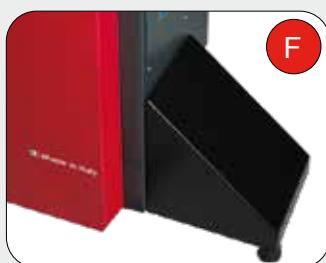
**(EN) STABILIZATION FOOT (OPTIONAL):** The standard supplied floor installation kit allows the machine to operate on wheels having maximum weight of 85 kg (187 lbs). To avoid fixing the balancer on ground, a stabilization foot KIT P is available on demand for a maximum machine wheel capacity of 50 Kg (110 lbs).
