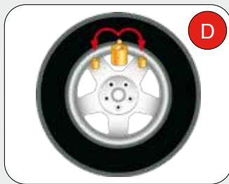
**(EN) HIDDEN WEIGHT AND SHIFT PLANE PROGRAMS (ALU P):** «Hidden Weight» subdivides the external adhesive weight in 2 parts to be positioned behind the spokes of the rim. The program «Shift Plane» calculates the balancing position to allow using commercial adhesive weights.
