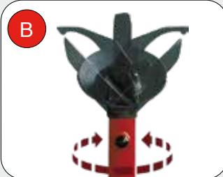
**(EN) TOOL-HOLDER ARM:** Tool-holder arm lifting and tool rotation are automatically achieved through the on-purpose control unit. The special semi-spherical shape of the bead breaker disc allows to obtain a better penetration between rim and tyre bead in order to avoid damaging the wheel.
