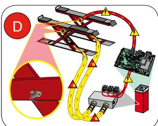
(EN) **RUNWAYS LEVELING SYSTEM:** Electronically controlled closed loop hydraulic runway leveling system for smooth lifting. Recesses of turntables and slip plates are also adjustable to ensure a perfect planarity of runways.
