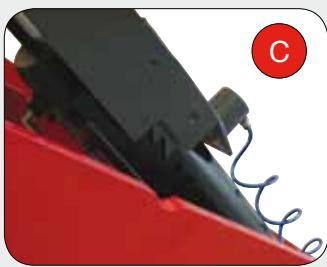
**EN** **MECHANICAL SAFETY LOCKS:** Automatic engagement of mechanical safety locks with automatic release system. Locks are adjustable and electronically controlled in order to grant the planarity of the lift in every working condition.
