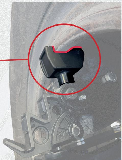
The unique clamping jaw profile has been designed so that it exactly reproduces the outer rim shoulder profile. The use of this accessory allows the wheel to be clamped on the machine chuck safely and quickly, ensuring a firm hold in both bead breaking directions.
