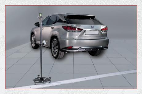
In this context of constant evolution, we created the new **SCE 310**, the equipment for the calibration of Radar sensors installed in the new generation vehicles of Toyota, Lexus, Mazda, Kia and Hyundai manufacturers.
